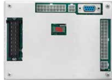
Main module inside the roof-top HVAC unit (145 x 104 x 31 mm)
